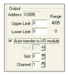
You should also select the analog output for the control output to be transferred to. This is done in the PID setup *Output* dialog shown here. The block of information in this dialog is "grayed-out" until the box next to *Auto transfer to I/O module* is checked. Once checked, the slot number defaults to "F" like the input, and the analog output channel can be selected.
