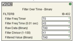
The rate at which the calculation is performed is specified by time in hundredths of a second (0.01 seconds) as the Filter Freq Time parameter. Note that this Timer instruction is embedded in the IBox and must NOT be used any other place in your program. Power flow controls whether the calculation is enabled. If it is disabled, the Filter Value is not updated. On the first scan from Program to Run mode, the Filter Value is initialized to 0 to give the calculation a consistent starting point.
